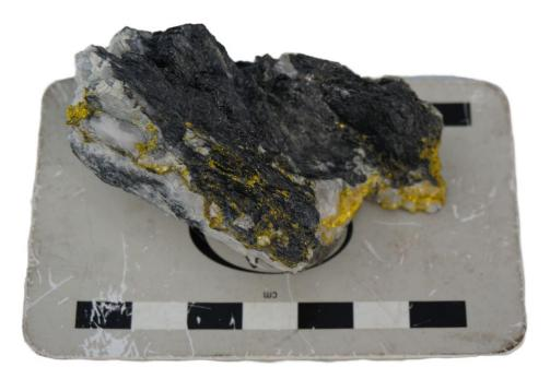
Figure 1 - Sample of in-situ bonanza bedrock gold - quartz vein in phyllite.
